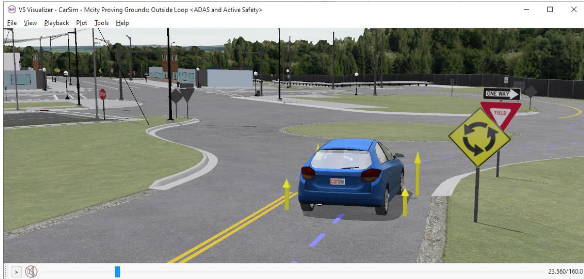
Figure 17. Complicated 3D ground geometry in Mcity is provided by VS Terrain.
